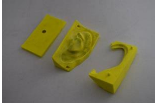
Fig. 8. 3D printed mold designed in Rhinoceros. (De-Rossi-Estrada et al, 2019).
