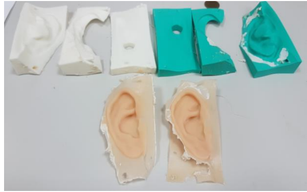
Fig. 13. Mold printed on the Prusa Mk3(left) and mold printed on the Ultimaker 3 Extended(right). (De-Rossi-Estrada et al, 2020).
