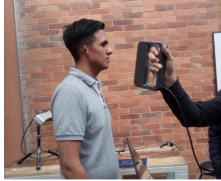
Fig. 10. Using the Isense 3D scanner. (De-Rossi-Estrada et al, 2019).
